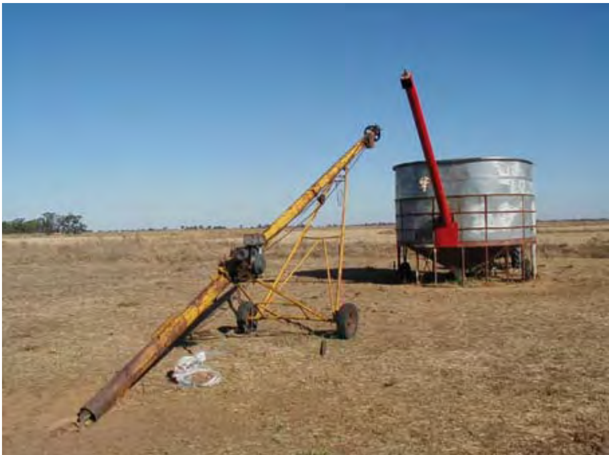
This type of machinery can fall on people and cause serious injury. Source: Agricultural Machinery Design and Operation Safety Study, Victoria, 2003–2006
