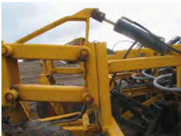
Examples of pinch and shear points that caused injury when being assembled or or maintained. Source: Agricultural Machinery Design and Operation Safety Study, Victoria, 2003–2006
