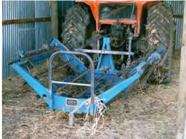
People have been injured by this type of machinery while undertaking maintenance activities. Source: Agricultural Machinery Design and Operation Safety Study, Victoria, 2003–2006
