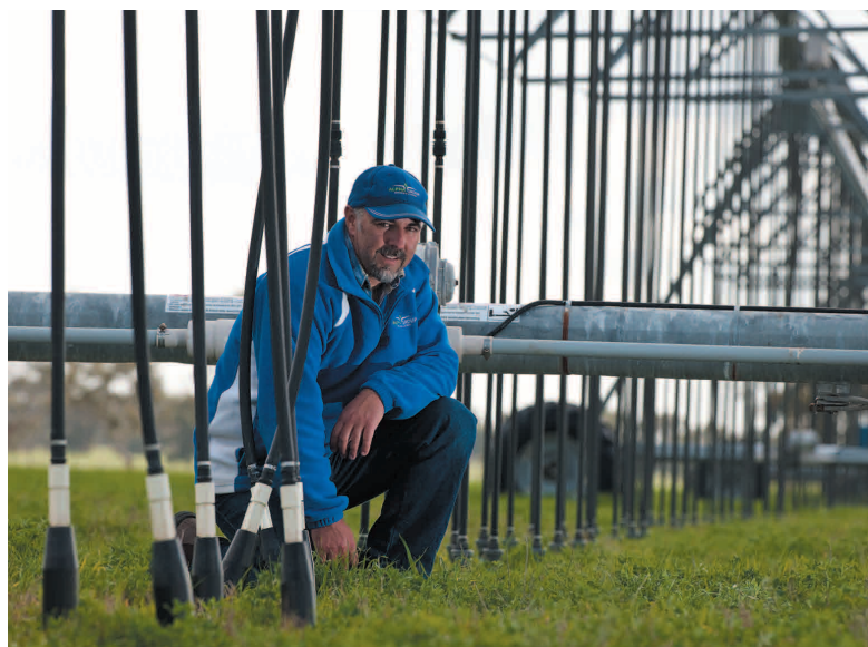
Researcher James De Barro showed 120% more profit per megalitre with drop tube irrigation compared with border check. Image courtesy of Coretext.
