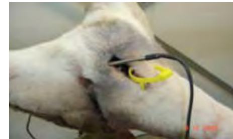
Figure 10. Temperature monitoring using a data logger
