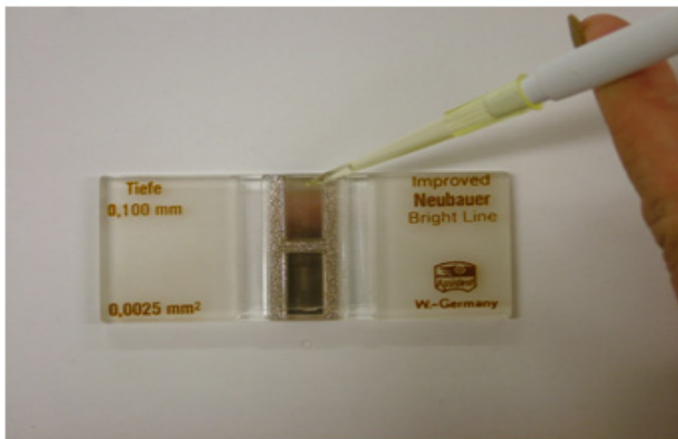
Figure 3: Inoculation of Improved Neubauer Counting Chamber to facilitate the counting of N. apis spores
