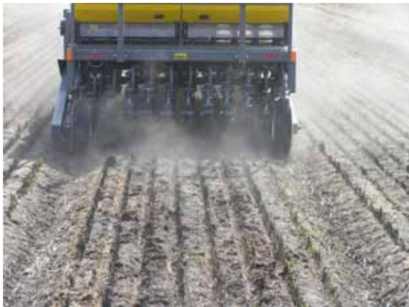
Figure 8. Stubble King No Till Drill sowing rice into bed layout
