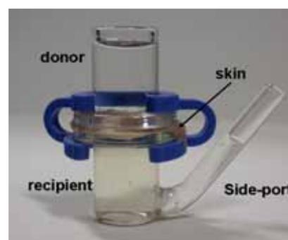
Figure 2. A typical diffusion cell
