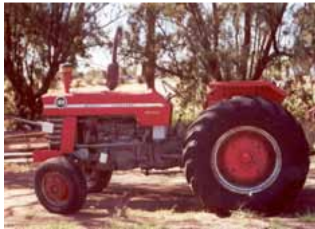
Tractor with open frame construction. Potential victims can fall or be standing in the area between the front and rear wheels.
