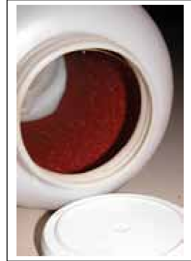
Figure 5 Glass paper lined tumbler.
