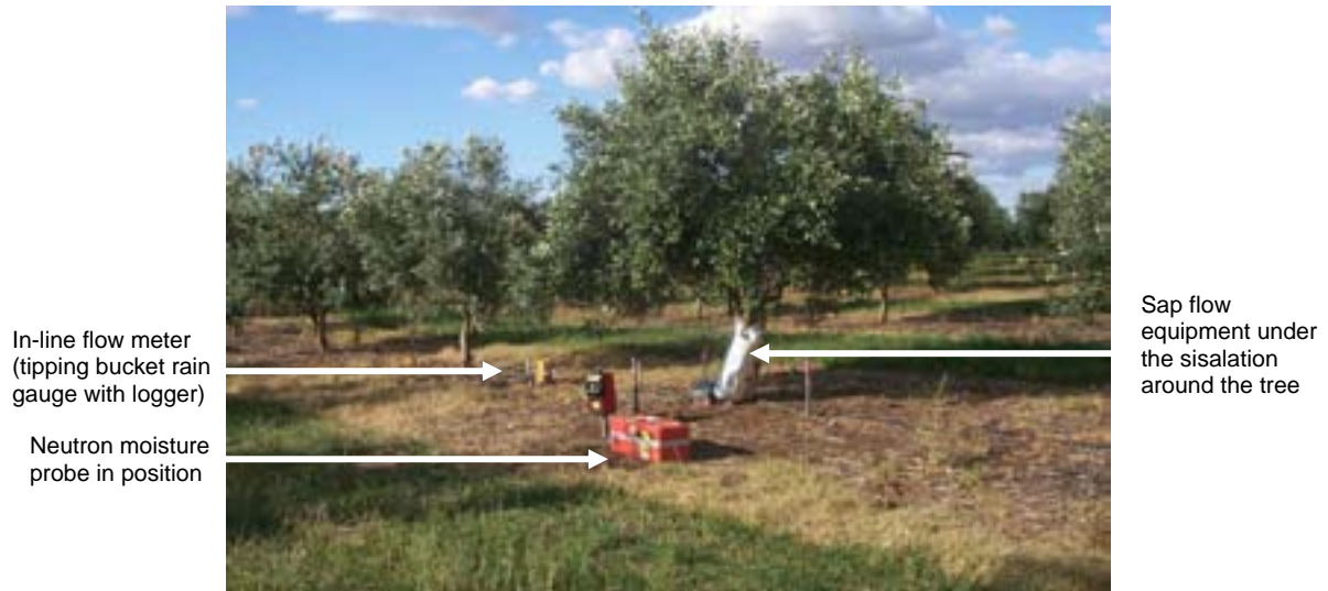
Photo 9 Instrumentation at the Waikerie site
