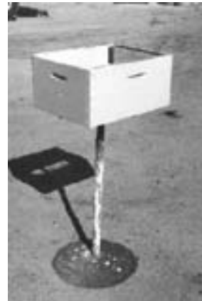
Photos 18 and 19. A revolving stand is useful when painting dipped supers which are very hot.
