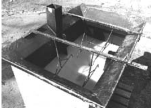
Photo 14. The clamps are used to keep the supers submerged in the molten wax.
