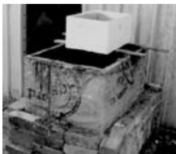
Photo 16. This vat is capable of dipping four supers at a time. Supers are removed from the wax and placed on two metal cross beams to allow excess wax to drain. The vat is partially insulated with aluminium insulation and bricks. Completion of the brickwork would greatly improve the insulation and prevent heat loss.
