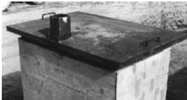
Photo 15. Wax dipping unit with lid in place.
